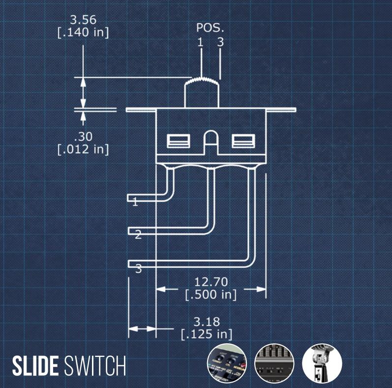
Slide switch utilizes a mechanical lever turning electrical current on and off. Depending on the number of positions available, the lever can move (slide)between an open or closed state. Compact in size, E-Switch offers Slide switches with multiple termination options. Slide switches are commonly used in computer server/peripheral equipment, instrumentation devices, test & measurement equipment and consumer electronics and household appliances.
