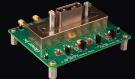
HiPer-D connector with size #8 opto-electronic contacts evaluation board
