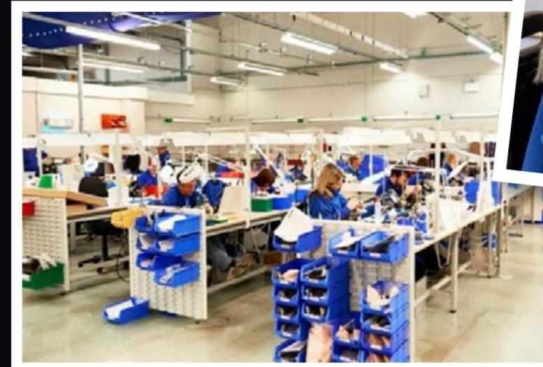
The Glenair Mansfield clean room assembly area is used for fabrication of laser, space, and satellite assemblies IAW ISO Class 8 -100,000 PPM
