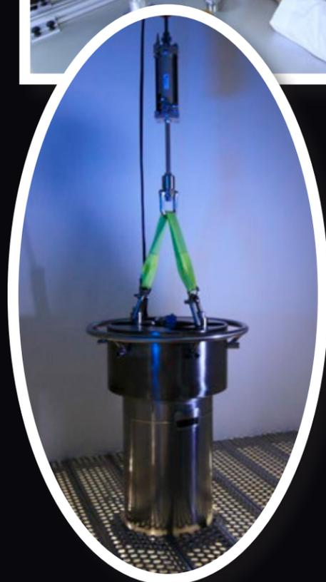
**LARGE PRESSURE VESSELS:** Built to accommodate complete cable assemblies, mated connectors, and customer-supplied subassemblies
