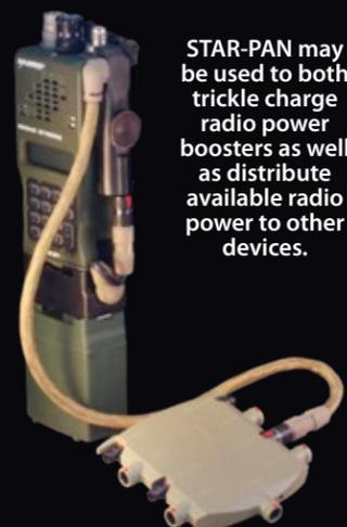
STAR-PAN may be used to both trickle charge radio power boosters as well as distribute available radio power to other devices.
