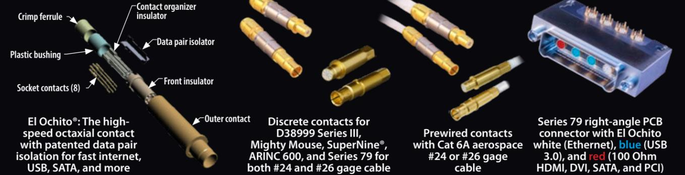
El Ochito®: The high-speed octaxial contact with patented data pair isolation for fast internet, USB, SATA, and more
