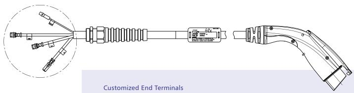
ITT Cannon EV solutions are available with a wide variety of customer specified end terminal options. The cables are effectively plug and play as minimal amends are needed at the customer site before deployment reducing cost, time and complexity.
