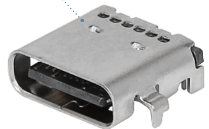
USB 3.2 Type-C Receptacle, Mid-Mount, 24 Circuit (217184 Series)
