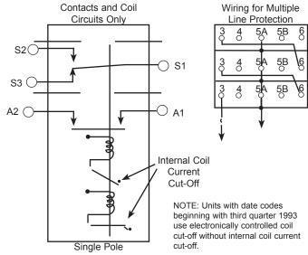
NOTE: Terminals 5A and 5B internally grounded to the mounting leg (s). Integrated wire termination (IWT) module accepts pin contacts P/N M39029/1-100 or -101. Use with insertion/extraction tool M81969/14-02.
