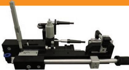
The P50/P100/P300/P350 machines can be supplied with modular insertion tools that allow the tooling to be quickly changed on the insertion head. A wide range of conversion kits for various TE Connectivity and non TE Connectivity products is available.
