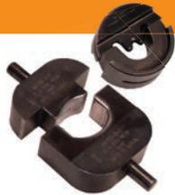
Our line of quality hydraulic tooling includes industry-standard 10,000 psi [68,950 kPa] and 8,200 psi [56,540 kPa] tool systems. The basic hydraulic tool system requires a pump, hose (multiple lengths are available with all configurations), crimp head, and crimp die. U-dies for a 10,000 psi hydraulic system are well suited for applications requiring a crimp force of up to 14 tons [125 kN]. For wire sizes requiring up to 33 tons [294 kN], TE offers crimp heads that are compatible with shank dies
